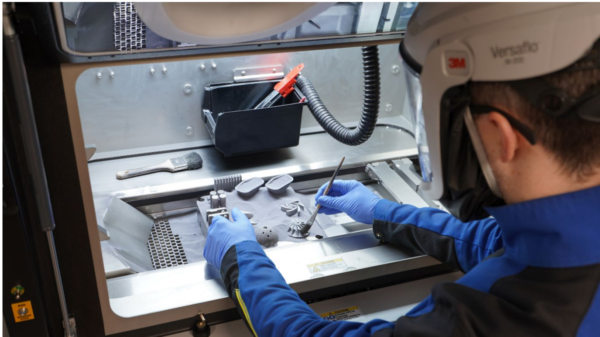
Tantalum components, manufactured using Croom Medical's TALOS™ additive manufacturing platform, being carefully unloaded post-print.
