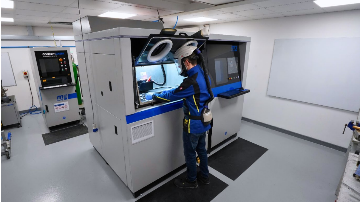
Croom Medical's additive manufacturing engineer operating the Colibrium Additive M2 Series 5 system, home to the TALOS™ platform.
